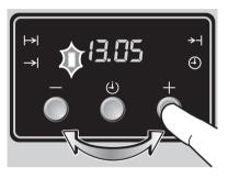
After approx. 5 seconds the display will revert to the time. The end time function indicator  $\rightarrow$  is illuminated.
